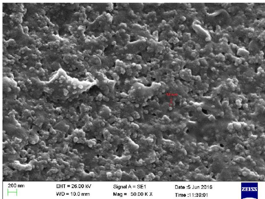
Fig. 5 SEM image of synthesized Ag NPs by aqueous extract of *Laurus nobilis* L. leaves.
