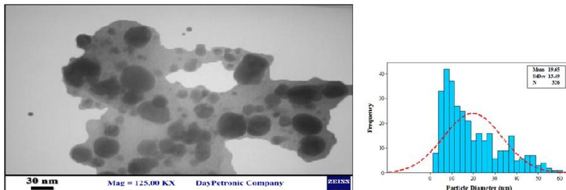
**Fig. 6** TEM image and corresponding particle size distribution histogram of synthesized Ag NPs by aqueous extract of *Laurus nobilis* L. leaves.
