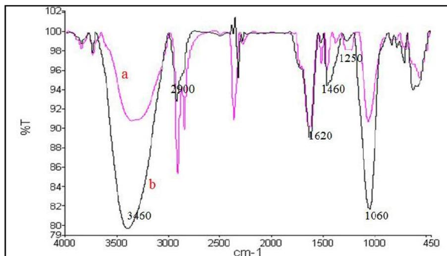
**Fig. 3** FT-IR analysis of (a) synthesized Ag NPs by *Laurus nobilis* L. leaves aqueous extract and (b) *Laurus nobilis* L. leaves aqueous extract.
