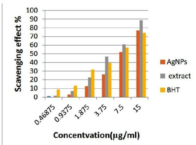
**Fig. 7** DPPH radical scavenging effect of *Laurus nobilis* L. aqueous extract and Ag NPs/extract suspension in comparison with BHT.
