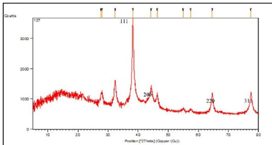
**Fig. 4** XRD patterns of Ag NPs synthesized by aqueous extract of *Laurus nobilis* L. leaves.
