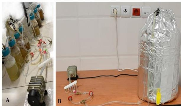
**Fig. 1** A: View of the one-liter bioreactor with aeration pump and sterile inlet and outlet air filters and fittings B: The 20-liter bioreactor with aeration pump, sterile inlet, and outlet air filters, electric agitator, and fittings.
