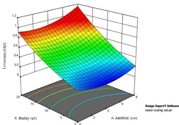
**Fig. 4** Three-dimensional display of the effect of carbon material (barley) (g/L) and aeration (L/min) on lovastatin production from *M. purpureus*. An increase in barley content increases lovastatin production. Increased lovastatin production at higher barley levels requires increased aeration.
