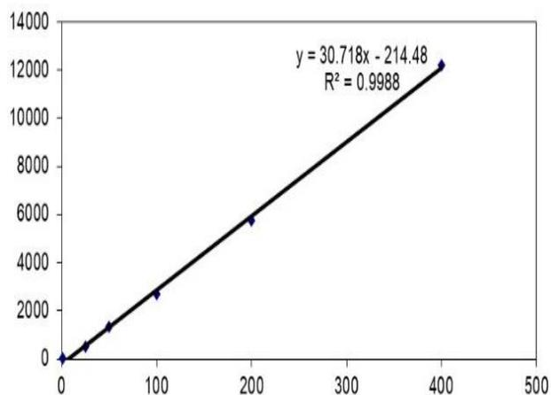
Fig. 4 The calibration line curve for trans-ferulic acid
