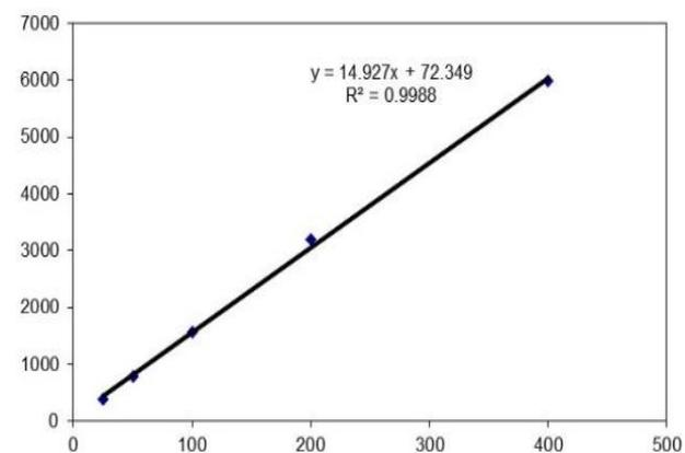
Fig. 3 The calibration line curve for quercetin
