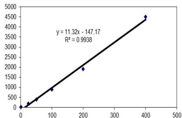
Fig. 5 The calibration line curve for eugenol
