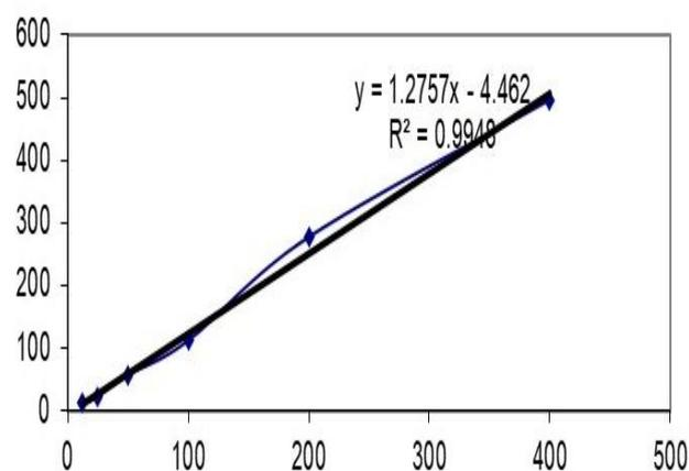
Fig. 2 The calibration line curve for gallic acid
