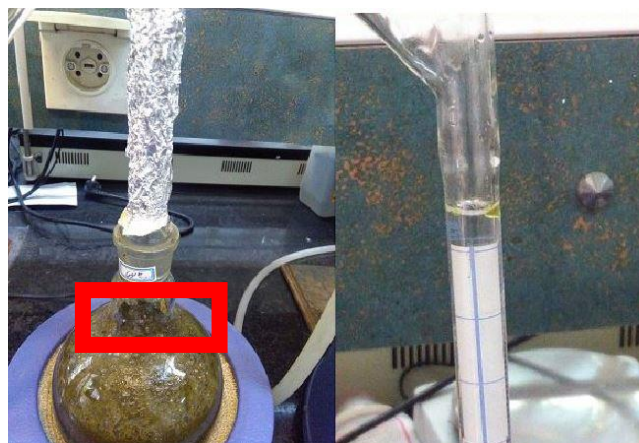
Fig. 1 Hydrodistillation of essential oil of T. farfara L. seeds using a Clevenger type apparatus.
