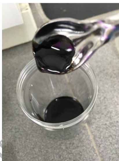
Fig. 2 The greenish oil extracted from SrB dried leaves using Soxhlet method in absolute ethanol
